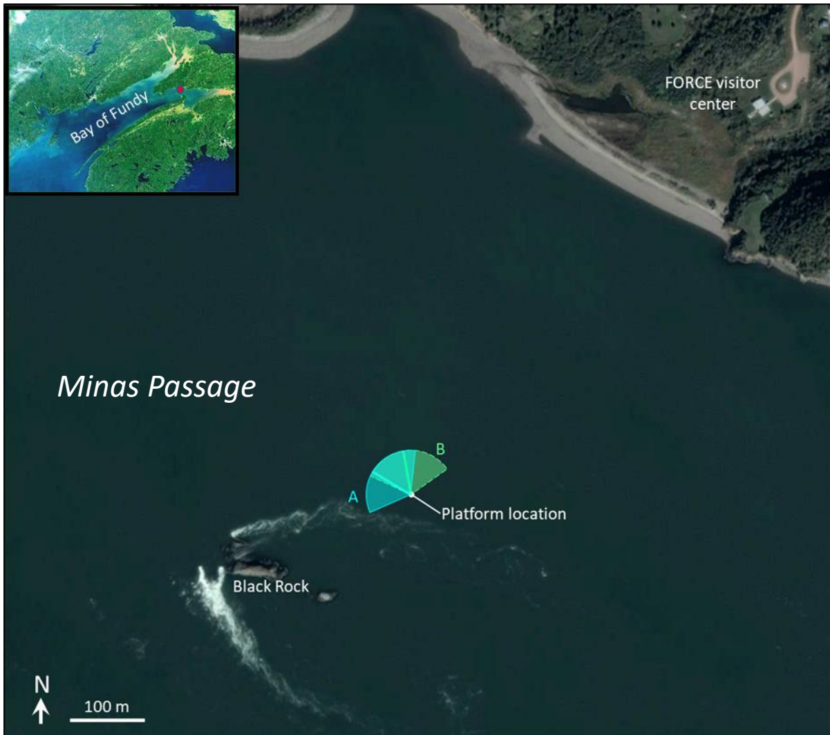
Figure 2. Location of platform in Minas Passage, 250m northeast of Black Rock. Shown are two different orientations of the Gemini sonar field of view (A and B). Eddies generated by Black Rock during ebb tide are visible at the surface.
