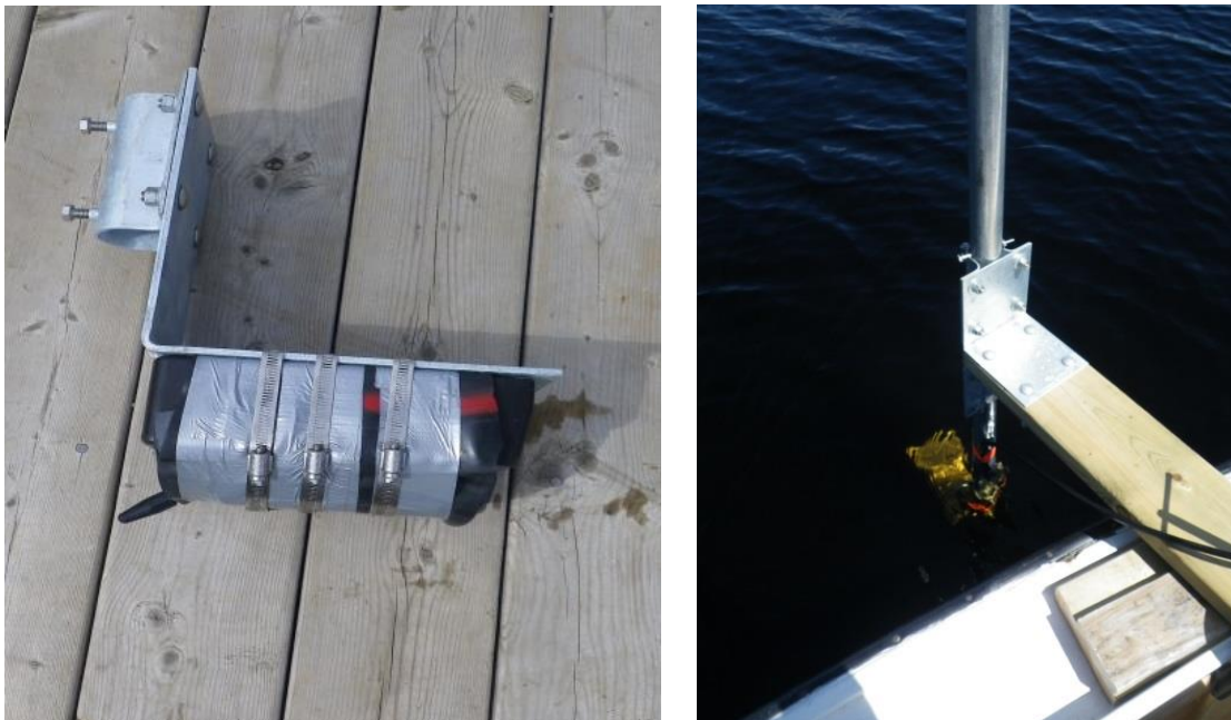
Figure 3. Tritech Gemini 720i attached to mounting bracket on dock prior to departure (Left). Gemini 720i mounted on adjustable pole structure and positioned perpendicular to the boat approximately 30cm below the surface (Right).
