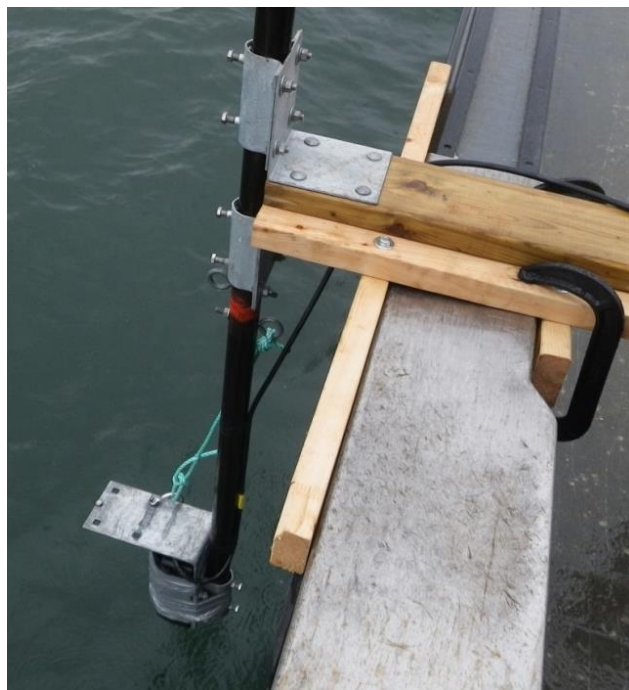
Figure 19. Pole mount clamped to the gunnel of the charter vessel. The Gemini 720i was positioned in a vertical viewing orientation during the Minas Passage drift test.
